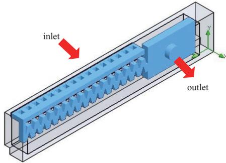
Fig. 4 Fluid subdomain of the emitter.
