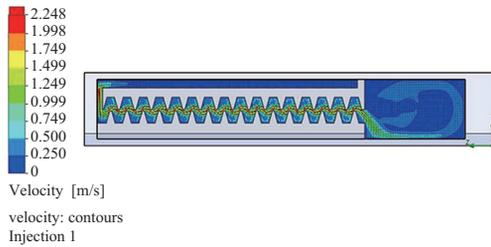
Fig. 6 Velocity contours of the emitter.
