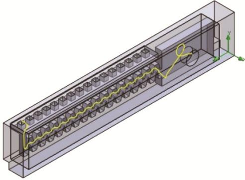
Fig. 8 Stream line in the emitter.
