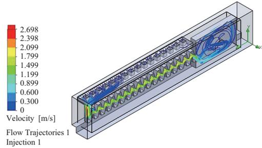
Fig. 5 Flow trajectories of the velocity.
