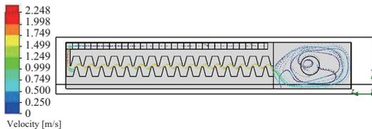
Fig. 13 Particle study top view of velocity trajectories (sw: 0.93).
