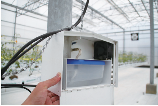
Fig. 1 Common psychrometer for greenhouse made by Priva B.V. in Netherlands.
